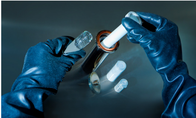
Assembling of a Na/NiCl 2 battery cell.
